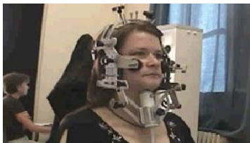
Figure 1: Speaker wearing headset and probe with VICON markers attached.
